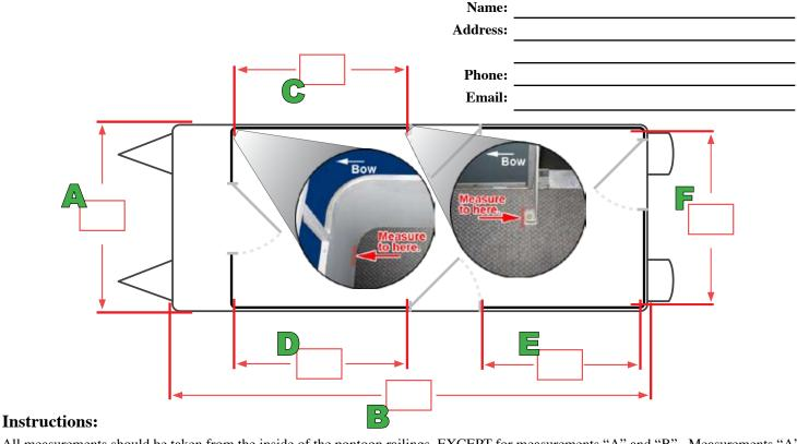
All measurements should be taken from the inside of the pontoon railings, EXCEPT for measurements "A" and "B". Measurements "A" and "B" are the overall width and length of your pontoon, and should be measured from the outer edges of the pontoon deck.
